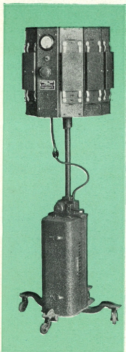
Uviarc Test Cabinet used for testing 20 to 60 samples of fabrics, yarn, paint, wood, etc.
